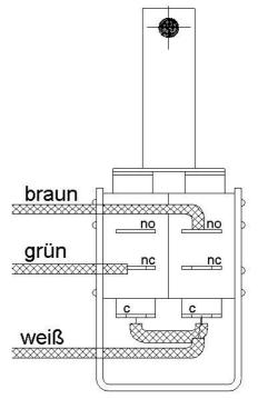
Im. 1: Terminal diagram door contact switch
