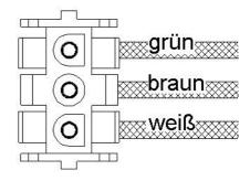
Im. 2: Terminal diagram connector (top view)
